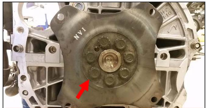
**Install new drive plate/flywheel bolts (ONLY if new bolts are included with the replacement engine)**
