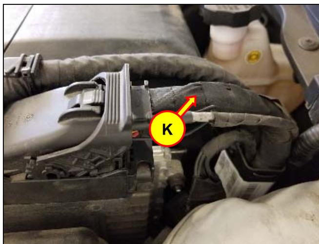
12. Cut off and discard the original knock sensor connector and fold the (2) original wires (L) from the original knock sensor connector back onto the original engine control wire harness and secure with tape.
